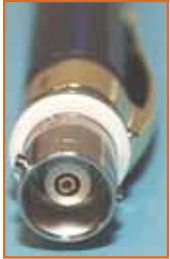
BNC connector for solid signal connection. Removeable connection for easy storage.
